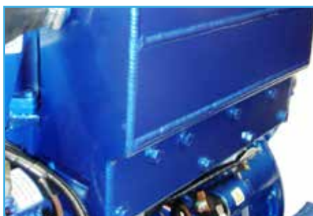
Water cooled manifold
