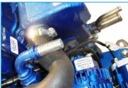
Hot water connections
